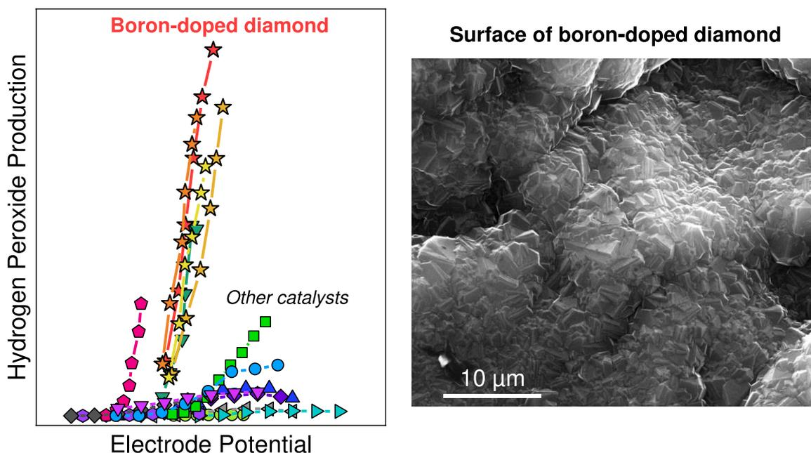
Performance of tailored boron-doped diamond (BDD) microfilms introduced by SOTON compared to other reported electrocatalysts in the literature for the WOR to produce H<sub>2</sub>O<sub>2</sub>
