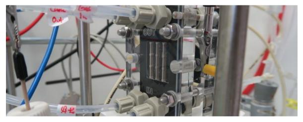
10 cm<sup>2</sup> electrochemical cell for water oxidation in test bench (Photo: Fraunhofer IGB 2020)
